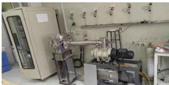
Fig.2. The PECVD device used for conducting the experiments.
